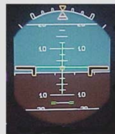
AT FLARE, WINGS LEVEL : In this case, the wings are at level, but the fog layer has a tilted base / surface of about 5^\circ . Outside visual perception is similar to the above illustration i.e. of a left 5^\circ bank.
