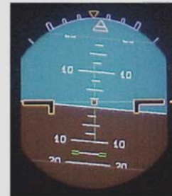
AT FLARE, LEFT BANK ( about 5^\circ ) : Notice the effect of the bank, the external perception indicates an inclined fog base / surface tilted with the aircraft bank.
